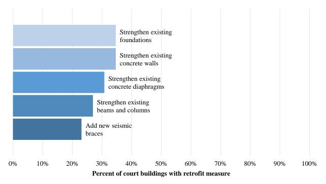
Figure 3. Common Retrofit Measures For the 26 Court Buildings in This Study
