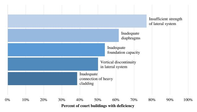
Figure 2. Common Seismic Deficiencies For the 26 Court Buildings in This Study
