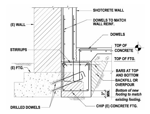
RETROFIT DETAIL 5: Sample Detail of Strengthening of Existing Beam as Collector
