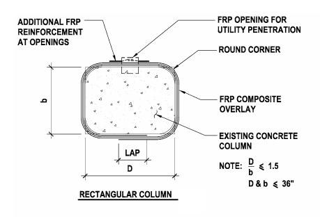
RETROFIT DETAIL 10: Sample Detail of Seismic Retrofit of columns
