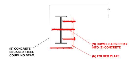
RETROFIT DETAIL 11: Sample Detail of Seismic Retrofit of Existing Concrete Encased Steel Coupling Beams
