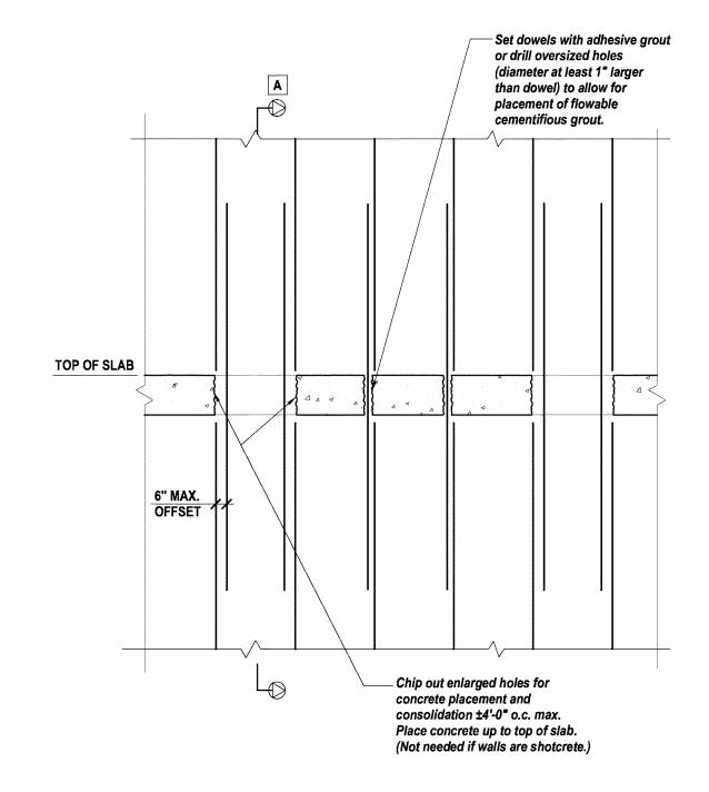
RETROFIT DETAIL 1: Sample detail of Strengthening of Existing Concrete Walls
