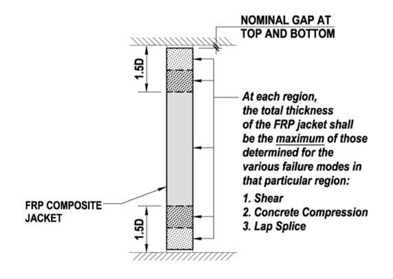
RETROFIT DETAIL 9: Sample Detail of Seismic Retrofit of columns
