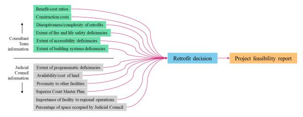
Figure 4. List of Factors Considered in Selection of Retrofit or Replacement Option
