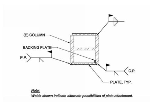
DETAIL 4: Box section at existing column (FEMA 547)
