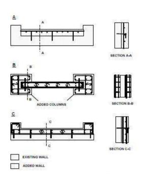
DETAIL 6 (Source: Aguilar, 1995): Conceptual Wall Retrofit With Shotcreting and/or Boundary Element Addition
