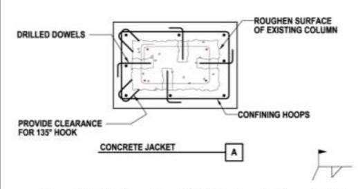
Figure 12.4.5-1: Concrete and Steel Overlays for Concrete Columns DETAIL 1: Column strengthening at basement (Source: FEMA-547)
