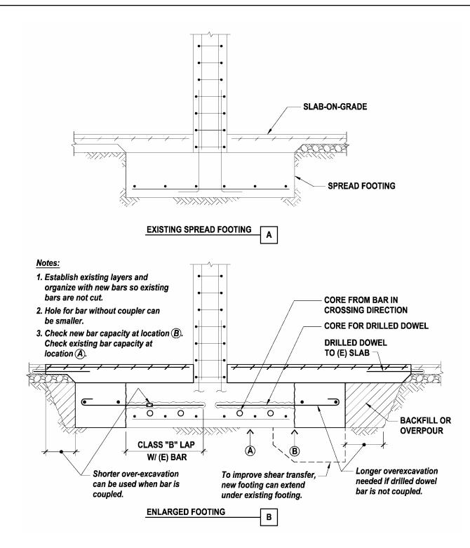
Figure 23.7.3-1: Enlarge Existing Spread Footing
