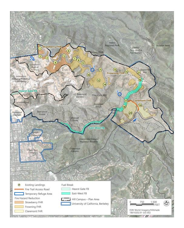
To develop the plan and select the project locations, the University used fuel models to predict fire behavior on the Hill Campus. The modeling considered factors such as predicted flame length, rate of spread, crown fire activity, and maximum spotting distance, along with
